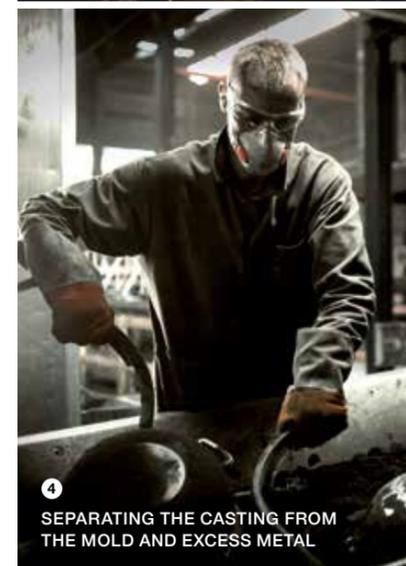
4 SEPARATING THE CASTING FROM THE MOLD AND EXCESS METAL
