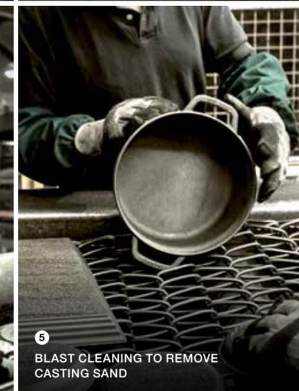
5 BLAST CLEANING TO REMOVE CASTING SAND
