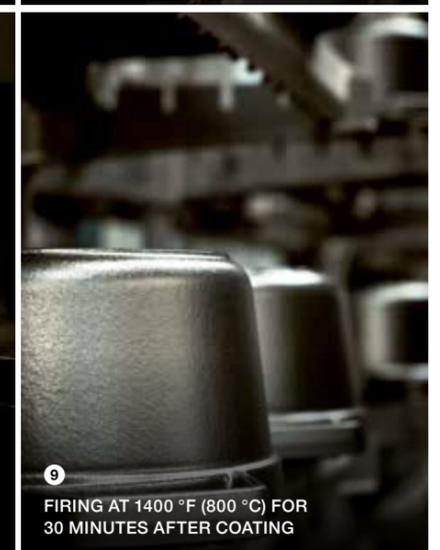
9 FIRING AT 1400 °F (800 °C) FOR 30 MINUTES AFTER COATING
